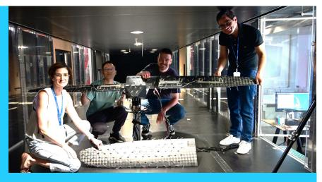
A key objective was validating the custom MCU-based DAQ system. Selected strain gauges were connected simultaneously to both the MCU and a commercial DAQ system, with the MCU demonstrating high signal fidelity, synchronization, and stability, closely matching commercial equipment.
